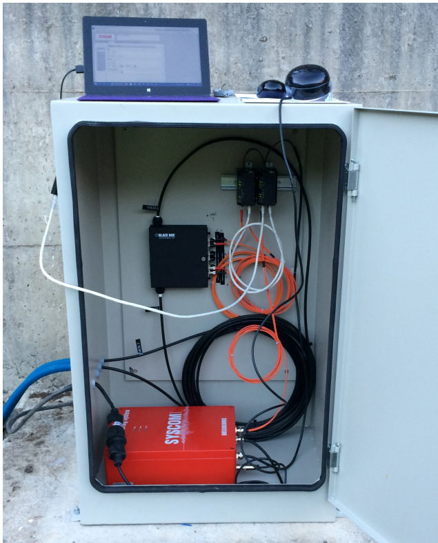
Figure 4. Horizontal mount MR3000DMS with GPS antenna at location ER4 in Evinos dam.
