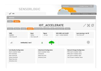
In addition, monitoring a change in the Cell-ID location is useful for devices that are not intended to be mobile after installation (e.g. vending machine, pumps, etc.). Knowing the exact location of devices and which MNO network is providing is crucial to controlling MNO roaming expenses as well as safeguarding against theft or vandalism
