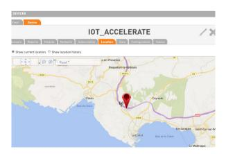
A Cell-ID geo-location service is proposed in order to locate or track a cellular-based device whenever the GNSS / GPS receiver signal is too weak or simply no receiver is available. Location history, geocoding and geofence services are then enabled.
